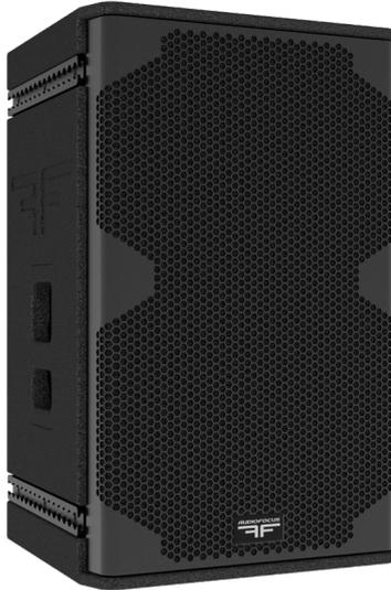
FRX 15a is a compact, powerful self-powered 2-way constant curvature loudspeaker, optimized for medium throw, high SPL live applications. FRX15a is a uniquely versatile building block for systems ranging from single top pole mounts to left/right, central cluster, or in the round setups. Typically used in horizontal ground stack configurations, FRX 15a can also be flown and its adjustable 80°x30° AF horn can be reconfigured quickly without the need for tools.
